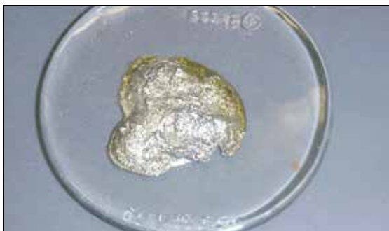
Fig. 67. Grease removed from an underfilled bearing shows shiny bearing metal debris.
